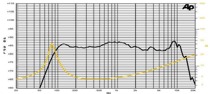
Frequency Response on 5.5 Lt @ 110 Hz Vented Box @ 1W, 1m
